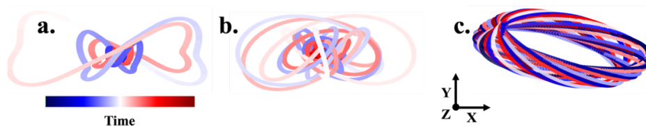
Figure 1. Ultrafast polarization induced in the hydrogen atom by our locally chiral field 1 a , total polarization the presence of the field. b , high-order components, resulting from filtering out the linear response in a . c , induced polarization after the pulse is gone.
