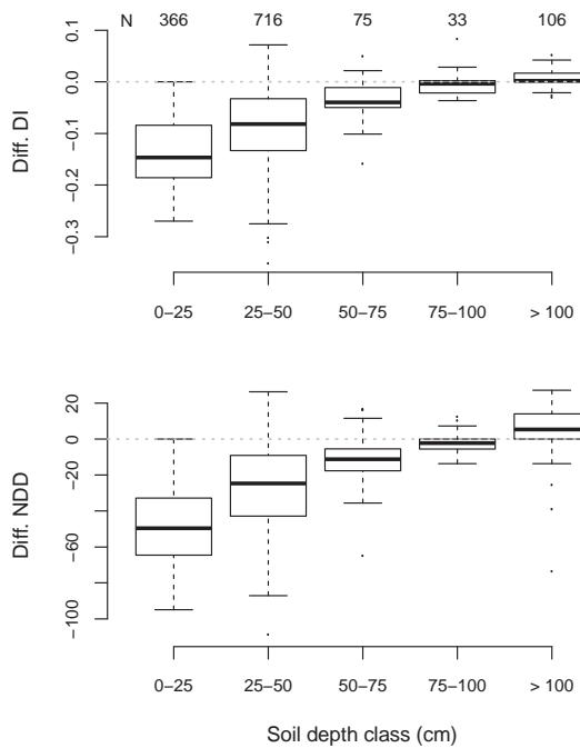
**Fig. 4.** Difference between drought stress values (DI and NDD) obtained assuming 100 cm soil depth for all plot records and drought stress values obtained using soil depth estimates available for three catchments (Fig. 1). N – Number of forest plots in each soil depth class.
