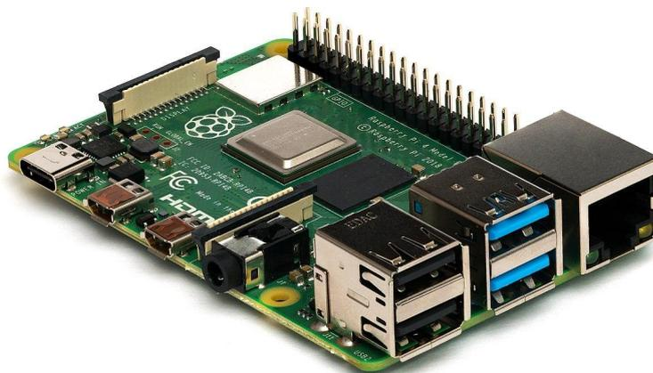
*Figura 4 - Raspberry Pi 4 Model B.
