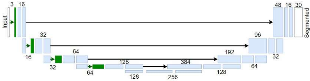
Figure 2.11: U-Net architecture model built for segmentation including 4 GDN layers (in green). Black arrows represent the skip unions. The model with only one GDN layer had only the first green layer. The model without GDN layers did not have any of the green layers. The consideration of the GDN layers only increases the number of parameters by an 1.8% in the case of the 4 GDN layers.
