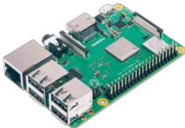
Figura 4.1: Raspberry pi 3B.
