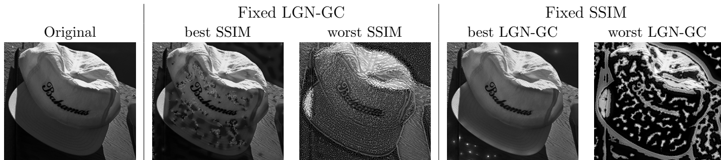
Figure 3: Comparison of SSIM and LGN-GC using MAD competition. Left: Original image. Middle: Maximally and minimally distorted images according to SSIM, with equal distortions according to LGN-GC. Right: Maximally and minimally distorted images according to LGN-GC, with equal distortions according to SSIM. Middle two images exhibit approximately equal perceptual quality (in agreement with LGN-GC), whereas the right two are noticeably different (in disagreement with SSIM).
