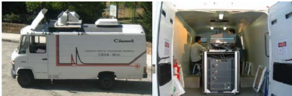
Figure 4.5 CIEMAT Mobile laboratory carrying LIDAR and related devices.
