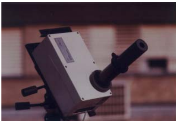
Figure 4.1. Licor 1800 Spectroradiometer. Direct irradiance measurements
