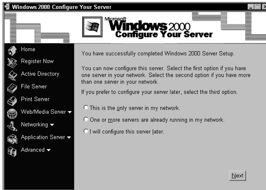
Figure 6-3: You can use Configure Your Server to start the Active Directory Installation Wizard.
