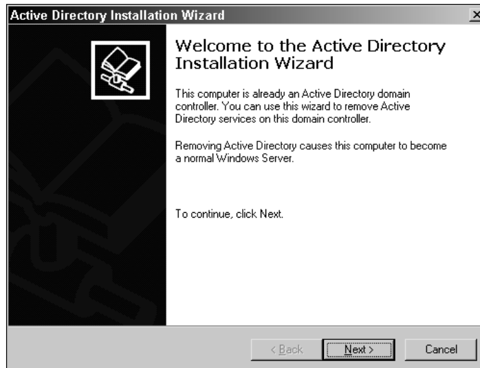
Figure 7-17: Removal of the Active Directory will demote this DC to a member server.
