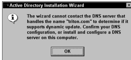
Figure 6-14: Click OK to automatically install DNS.
