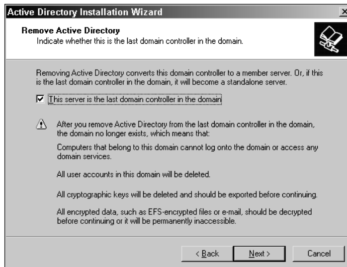
Figure 7-19: Click the check box if this is the last DC in the domain.
