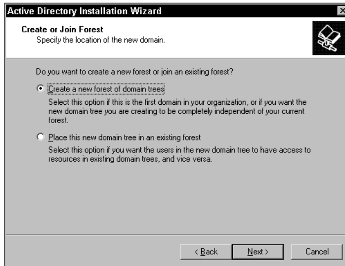
Figure 6-9: Click the create a new forest radio button and then click Next.
