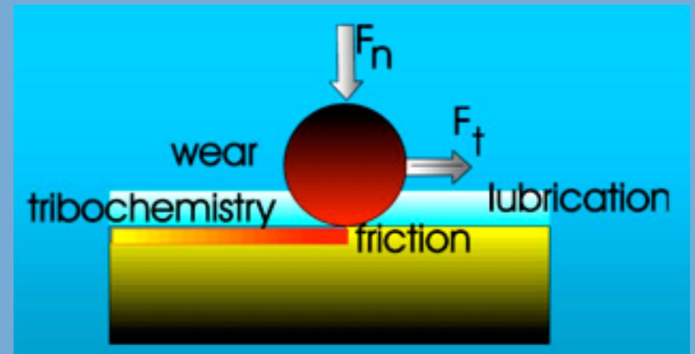
$$W_{\text{total}} = W_{\text{mechan}} + W_{\text{corr}} + W_{\text{synerg}}$$
