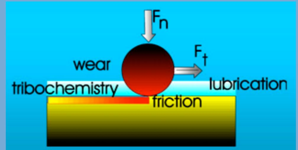
$$W_{\text{total}} = W_{\text{mechan}} + W_{\text{corr}} + W_{\text{synerg}}$$
