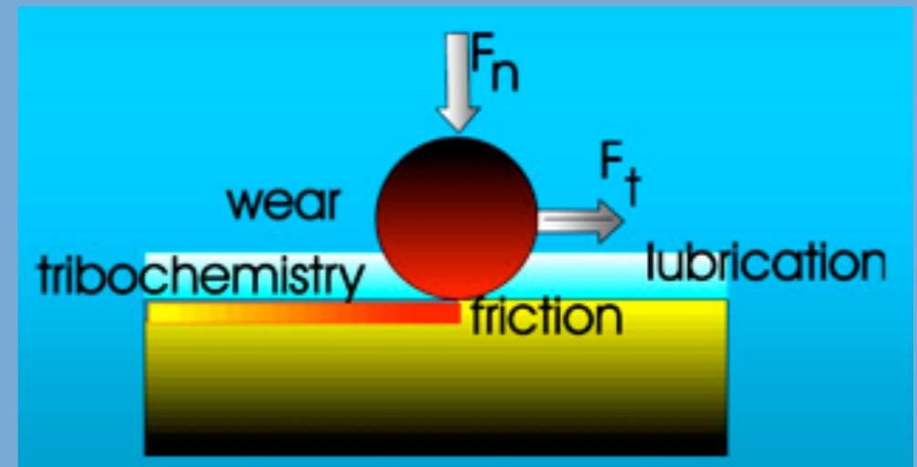
$$W_{\text{total}} = W_{\text{mechan}} + W_{\text{corr}} + W_{\text{synerg}}$$
