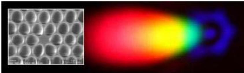
Supercontinuum generation using photonic crystal fibers
