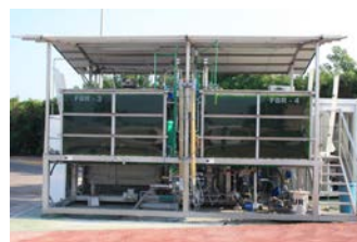
Image of the pilot plant for the cultivation and harvesting of microalgae
