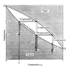
**<u>Figure 1.</u>** Phase diagram (liquid-vapor) temperature versus composition corresponding to an ideal mixture with A more volatile than B.
