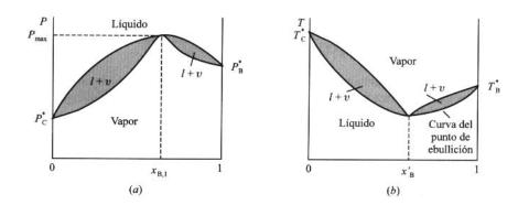
**<u>Figure 2</u>**. (a) Liquid-vapor phase diagram, pressure versus composition, with a maximum. (b) The corresponding diagram of temperature versus composition with its minimum.
