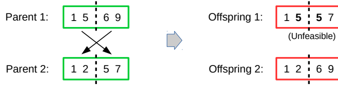
Figure 3: Usual single-point crossover. First offspring is not a feasible solution.
