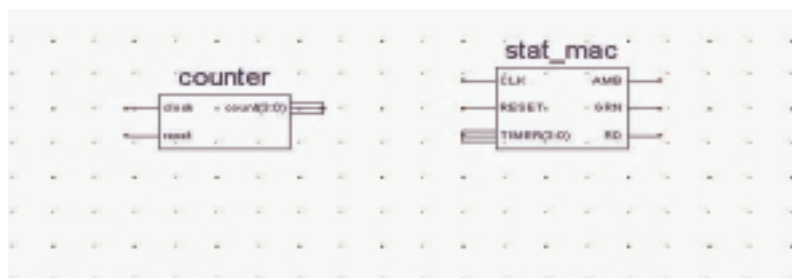
FIGURE 4-34: CLOSE-UP OF COUNTER AND STATE MACHINE SYMBOLS
