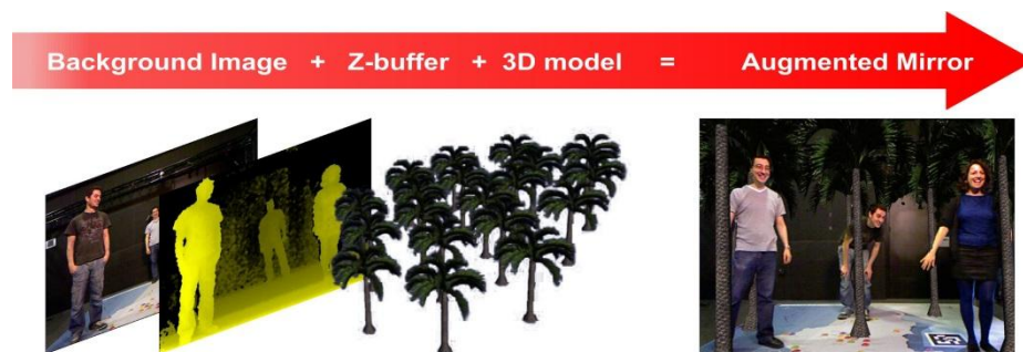
Fig. 2. Augmented reality scene composition using depth information.
