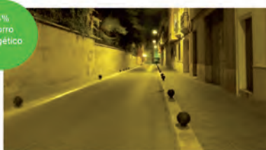
SON100W PC (120W medidos) H:6m, S:21m, Ancho 3m Ehmed 19lux, Uo =0.3 Ra 20 IRC: 25; Tc 2100K
