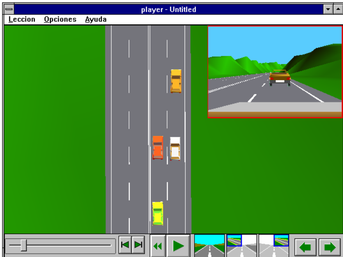
Figure 6: View of the player window in the PC no-texture version. The control bar is seen below; a main view (bird's eye) and the right auxiliary window with a from view from the white car are shown
