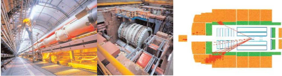
Figure 2: HERA: Accelerator (left), detector (center) and image of collision (right). Electron enters from left and bounces back violently. Proton from right has its quarks produce particles that shoot off to bottom left.
