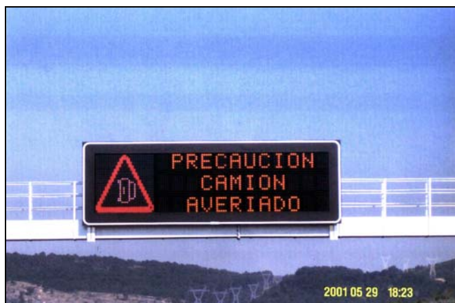
Fig. 1(b) – VMS-panel containing data
