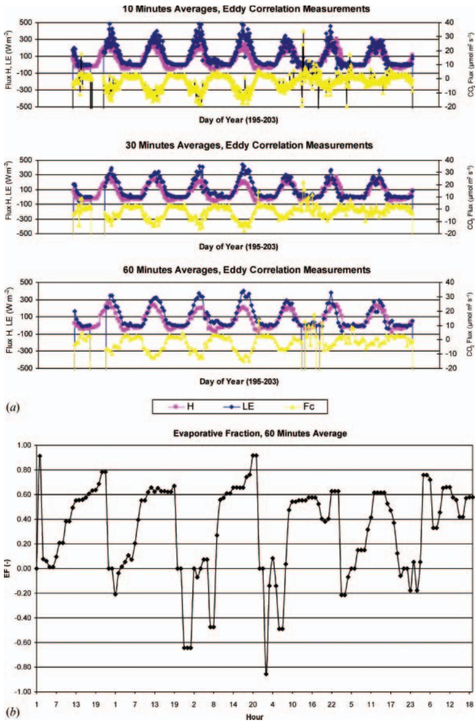
Figure 5. (a) Time-averaged sensible heat flux (H), H<sub>2</sub>O (LE) and CO<sub>2</sub> (Fc) fluxes and (b) time-averaged evaporative fraction (EF) measured with the eddy correlation station in SPARC 2004.
