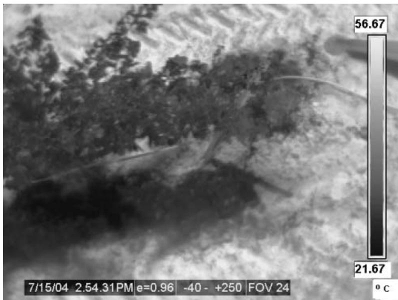
Figure 12. Radiometric temperature of the vineyard measured with an FLIR thermal camera in SPARC 2004. The spatial dimension of the image is approximately  $8\text{ m} \times 6\text{ m}$ .
