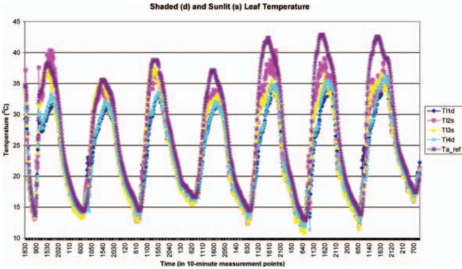
Figure 10. Leaf temperatures measured with thermal couples attached to the back of leaves in SPARC 2004. T11d and T14d were for shaded leaves, T12s and T13s were for sunlit leaves,  $T_{a\_ref}$  is also shown as a reference.
