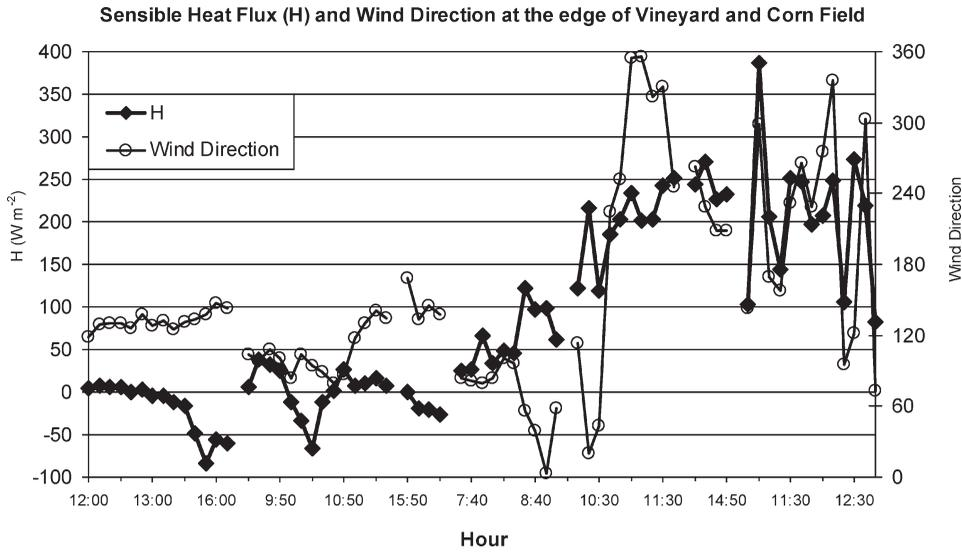
Figure 6. Time-averaged sensible heat flux measured with a 3D sonic anemometer at the corn–vineyard edge in SPARC 2004 (code 1 in figure 1 and table 1; north is set at 0°).
