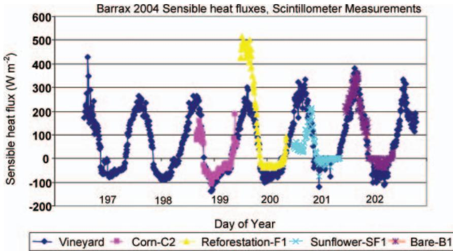
Figure 4. Sensible heat flux in SPARC 2004 (measurements made with scintillometers over different fields. See tables 1 and 2 for field code).
