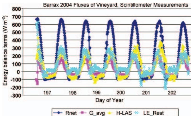
Figure 3. Energy balance components in the vineyard in SPARC 2004. Rnet, net radiation;  $G_{avg}$ , average soil heat flux;  $H_{LAS}$ , sensible heat flux;  $LE_{Rest}$ , latent heat flux estimated as residual of the energy balance.
