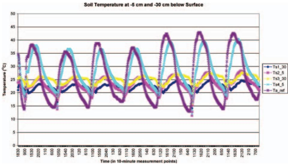
Figure 8. Soil temperatures measured with thermal couples at two levels in SPARC 2004. Ts1\_30, Ts2\_5, Ts3\_30 and Ts4\_5 are 30, 5, 30 and 5 cm below the surface, respectively; Ts1\_30 and Ts2\_5 are under the vine, while Ts3\_30 and Ts4\_5 are in the middle of the row; Ta\_ref is the reference air temperature measured at the eddy correlation station as shown in figure 5.
