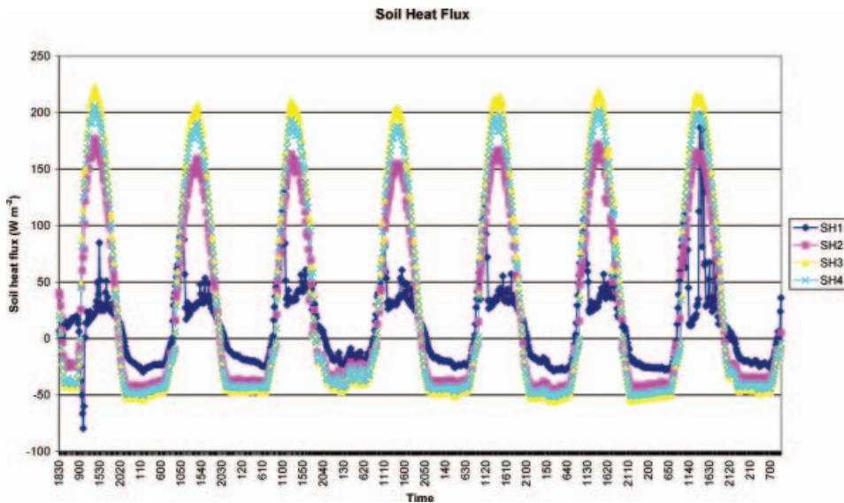
Figure 7. Soil heat fluxes in SPARC 2004. Soil heat flux plates SH1 and SH4 were in the shade; SH2 and SH3 were in the sunlit areas.
