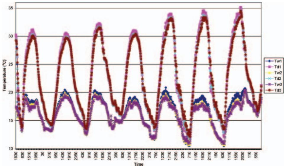
Figure 9. Air temperature and humidity measured at three levels. Tw is the wetbulb and Td the drybulb temperature; Tw1 and Td1 were set at a height of 0.65 m, Tw2 and Td2 at 1.65 m, and Tw3 and Td3 at 3.0 m.
