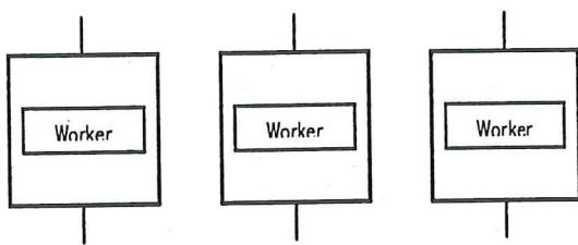
This is the faster and more scalable configuration. It is simply three pipelined channels each one of them working on a different colour co-ordinate from the same image. It is only convenient to the one-stage algorithm since the workers are not allowed to communicate partial results. Consequently, there are no delays.
