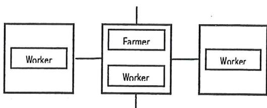
The *farmer* distributes the external information to the *workers*, co-ordinating communication between them and combining results. Each worker analyse a colour feature searching for clusters in the first stage and classifying one third of the total image in the fine stage.
