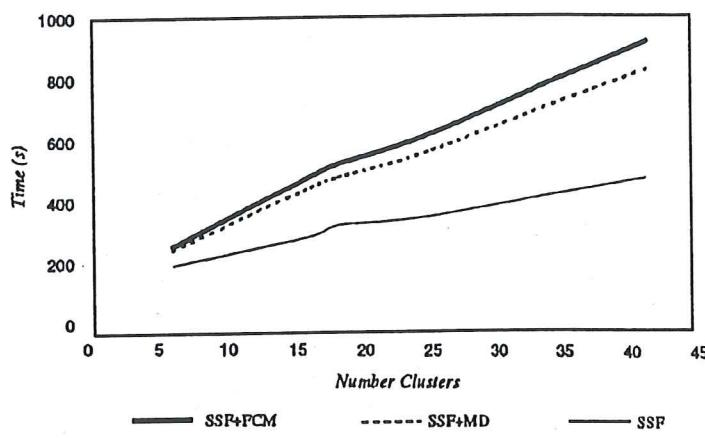
The sequential execution times of the proposed and the original algorithms are compared here. The test has been carried out with images leading to an increasing number of colour clusters. Time execution rates for algorithms using FCM and MD (minimum distance) strongly rely on the number of clusters. Total execution time only depends on the processor model used (transputer T805) and it must not be considered a characteristic.
