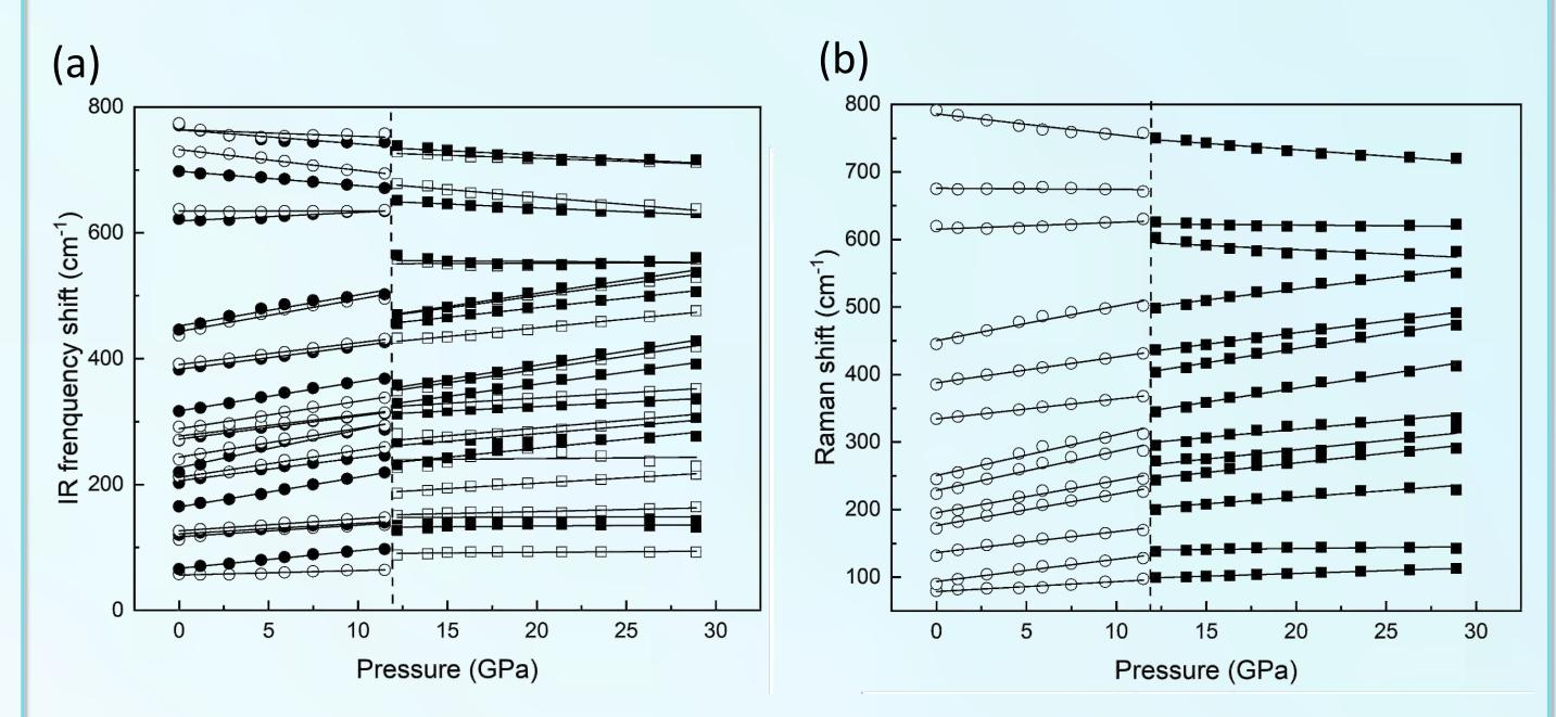
(a). Calculated pressure dependence of the Raman and IR-active modes (A and E1 modes, filled and empty symbol are used for E1 and A modes, respectively). (b) calculated pressure dependence of Raman-active modes only (E2 mode).
