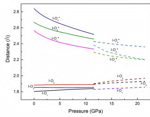
Calculated pressure dependence of I-O bond distance, solid line is for LP and dash line is for HP phase
