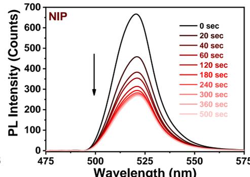
PL Intensity is very sensitive to the adsorption of NO<sub>2</sub>-Compounds at CsPbBr<sub>3</sub> PVK
