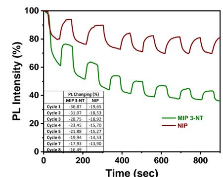
The analyte adsorption on the sensor surface is a reversible process
