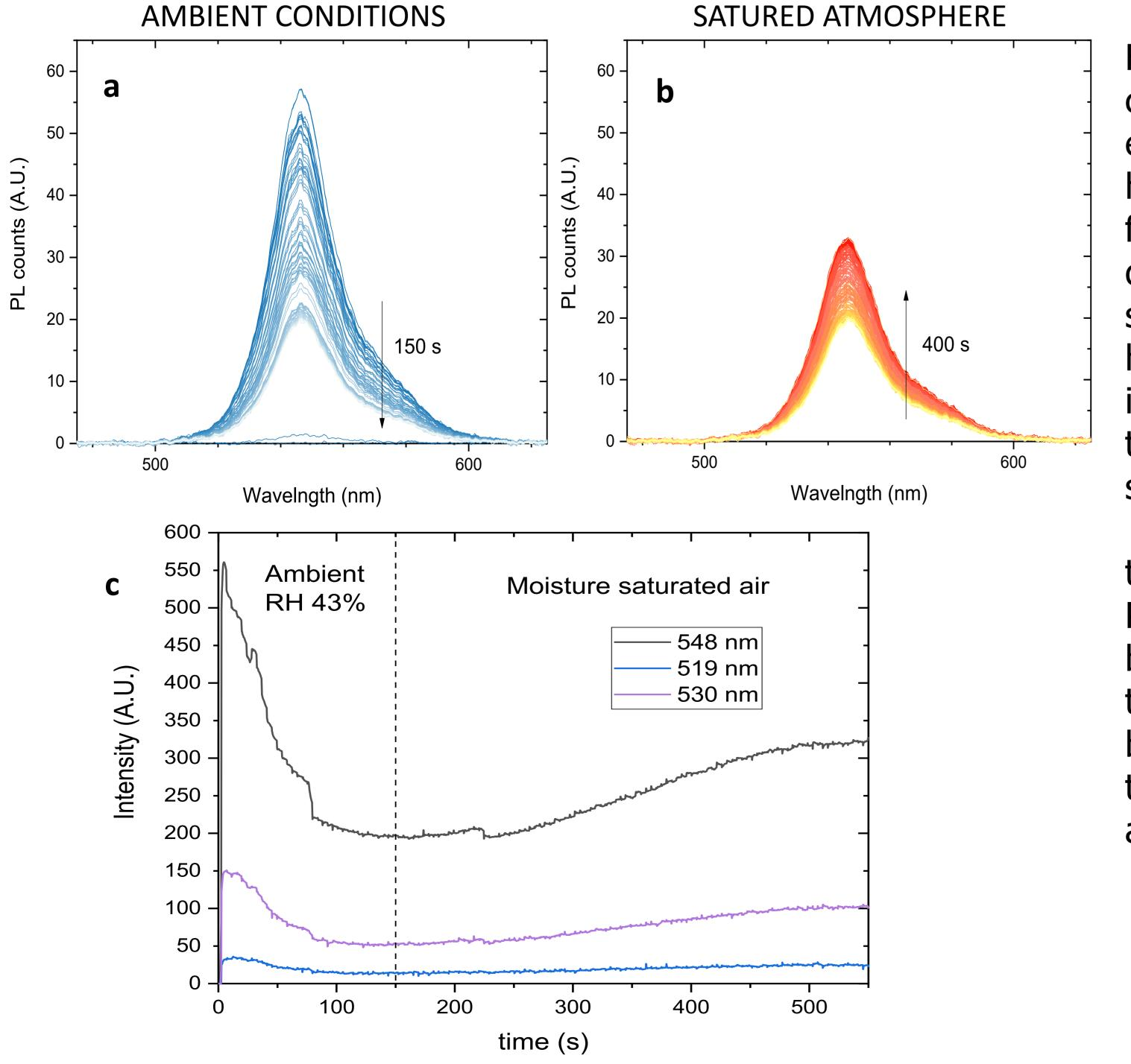
First, in ambient conditions, when laser excites the sample, a high PL signal appears, followed by a slight decrease and final stabilization (**a**). Under high humidity, the PL increases and reaches the stabilization stabilized (**b**). To gain insight of this trend, we measure the PL of three specific bands as a function of time (c) where 548 nm band is associated with the maximum absorption.
