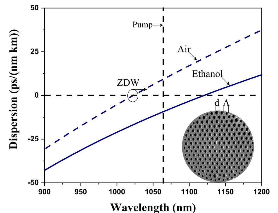
The PCFs employed during the experiments has the following fabrication parameters:  $d/\Lambda=0.75$  and  $\Lambda=3.9$  µm.
