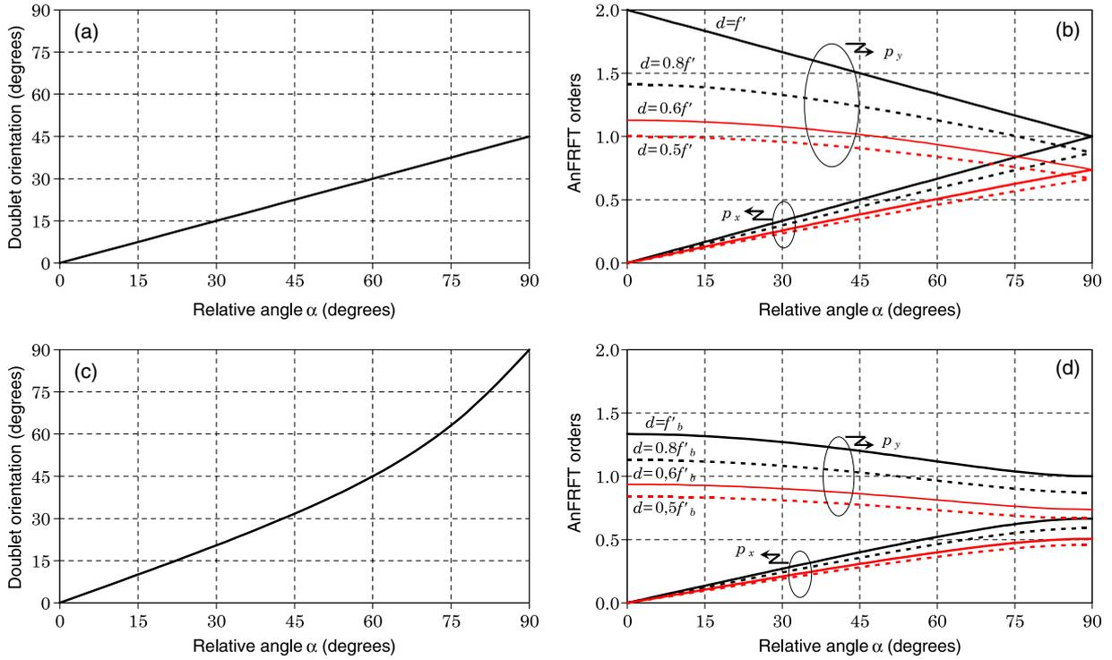
**Figure 8.** Orientation  $\varphi$  of the equivalent anamorphic doublet (a)–(c) and anamorphic fractional orders (AnFRFT orders)  $p_x$  and  $p_y$  (b)–(d), as a function of the relative angle  $\alpha$  between the two cylindrical lenses. (a) and (b):  $f'_a = f'_b \equiv f'$ . (c) and (d):  $f'_a = 2f'_b$ . Fractional orders are calculated for propagation distances  $d = f'$ ,  $d = 0.8f'$ ,  $d = 0.6f'$  and  $d = 0.5f'$ .
