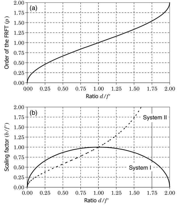
**Figure 3.** Evolution of the fractional order  $p$  and the scaling factor  $b$  as a function of the ratio  $d/f'$  in the two FRFT Lohmann systems in figure 2.
