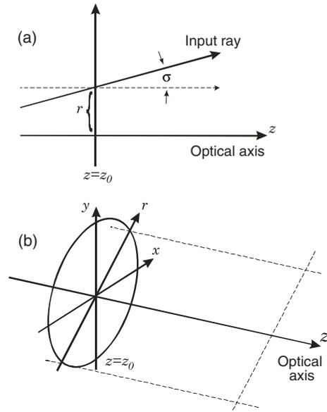
**Figure 1.** Coordinates for the ray matrix formalism. Input rays in rotationally symmetric systems are characterized by the height  $r$  and the angle  $\sigma$  they cross with respect to the optical axis.
