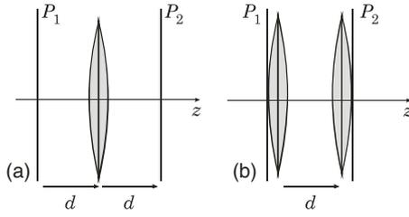
**Figure 2.** Two Lohmann fractional Fourier transform systems: (a) propagation–lens–propagation, (b) lens–propagation–lens.
