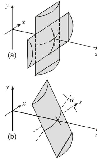
**Figure 4.** (a) Anamorphic lens with curvatures along the  $x$  and  $y$  directions. (b) Cylindrical lens with arbitrary orientation.
