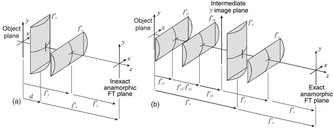
Figure 5. Inexact (a) and exact (b) anamorphic Fourier transformers.
