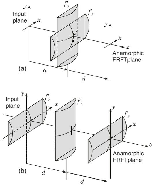
**Figure 6.** Anamorphic FRFT transform system in the  $x$ - $y$  directions.
