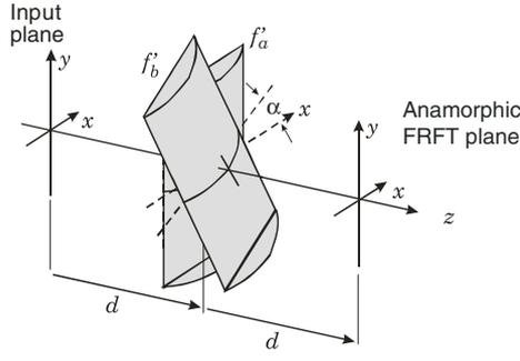
**Figure 7.** Cylindrical non-orthogonal doublet, and its application to perform an anamorphic fractional Fourier transformer with tunable fractional orders.
