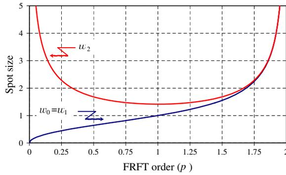
**Figure 6.** Evolution of the beam spot size at the beam waist ( $w_0$ ) and at the two mirrors ( $w_1$  and  $w_2$ ) as a function of the round trip FRFT order in a half-symmetric resonator. The spot size is represented in units of  $\sqrt{L\lambda/\pi}$ .
