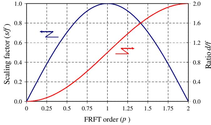
**Figure 2.** Evolution of the normalized scaling factor  $s/f$  and the ratio  $d/f$  as a function of the FRFT order ( $p$ ) in a Lohmann propagation–lens–propagation system.
