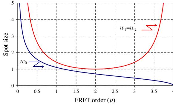
**Figure 5.** Evolution of the beam spot size at the beam waist ( $w_0$ ) and at the two mirrors ( $w_1$  and  $w_2$ ) as a function of the round trip FRFT order in a symmetric resonator. The spot size is represented in units of  $\sqrt{L\lambda/\pi}$ .
