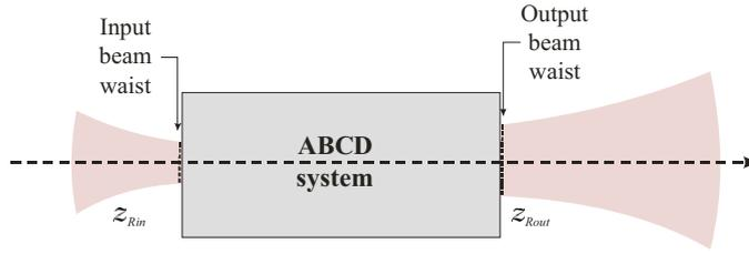
**Figure 1.** Optical system performing a Gaussian beam waist-to-waist transformation.
