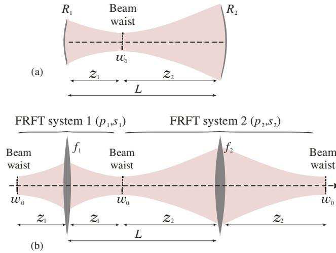
**Figure 3.** (a) Scheme of the optical resonator and its Gaussian mode. (b) Equivalent system composed of two Lohmann FRFT systems.
