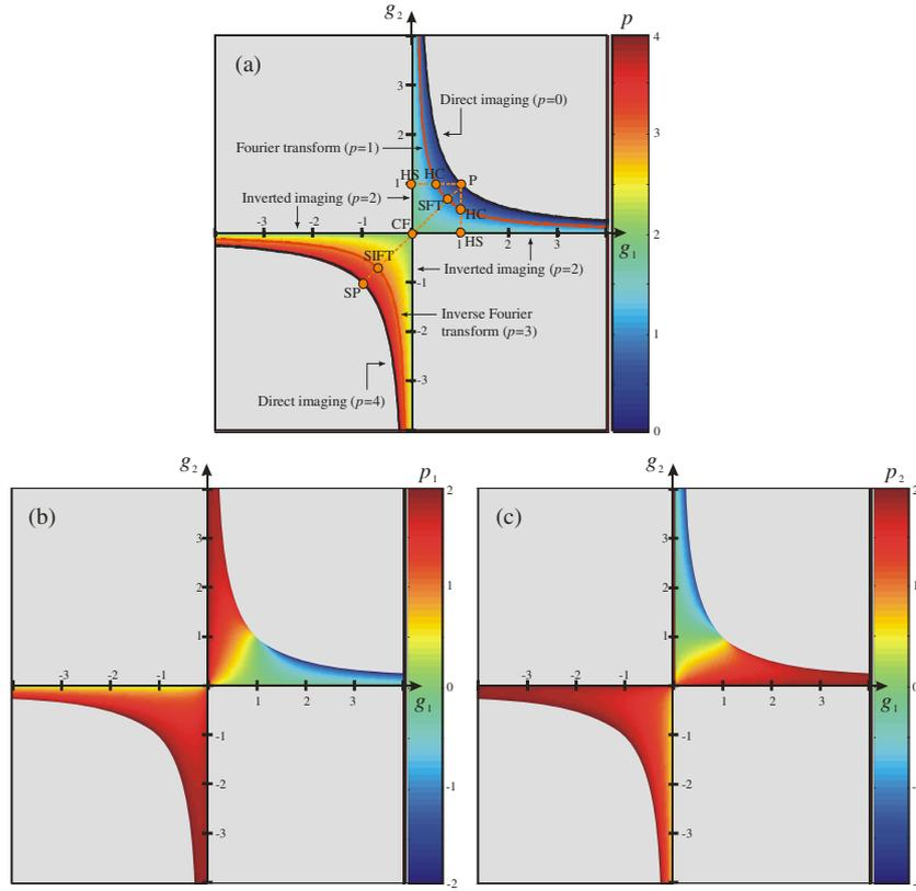
**Figure 4.** (a) Resonator's stability diagram and identification of FRFT curves. Some well-known resonators are indicated: P: planar; CF: confocal; SP: spherical; HC: hemi-confocal; HS: hemi-spherical; SFT: symmetrical direct Fourier transform resonator; SIFT: symmetrical inverse Fourier transform resonator. The FRFT orders of each subsystem are represented in the diagram in (b)  $p_1$  and (c)  $p_2$ .
