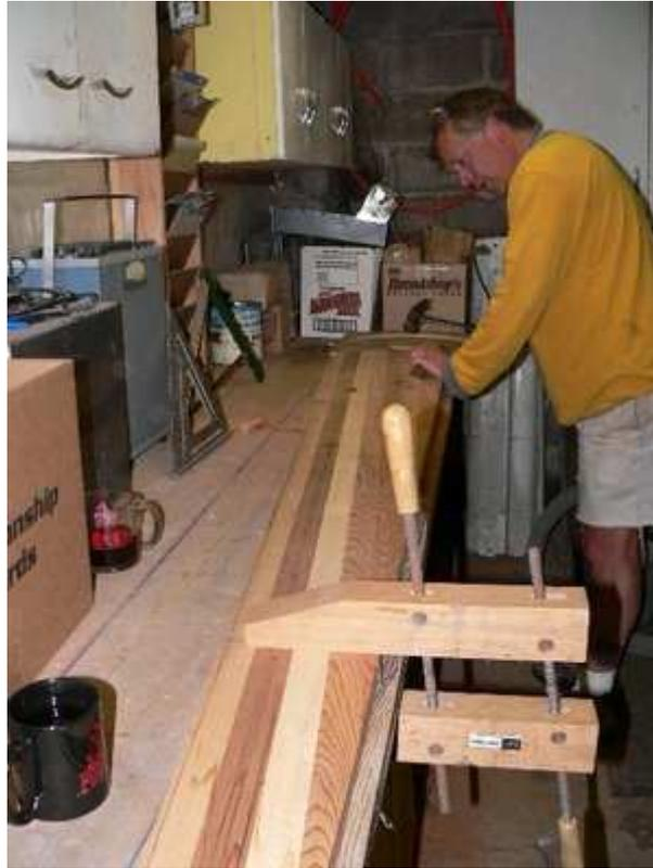
**Clay from the MREA uses a mallet and chisel to remove the chunks that were kerfed with the bowsaw.**
