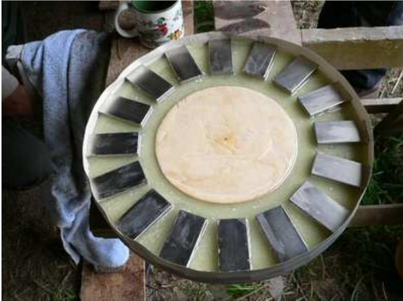
**A BIG magnet rotor for the 15 foot wind turbine. Danger, Will Robsinson!**
