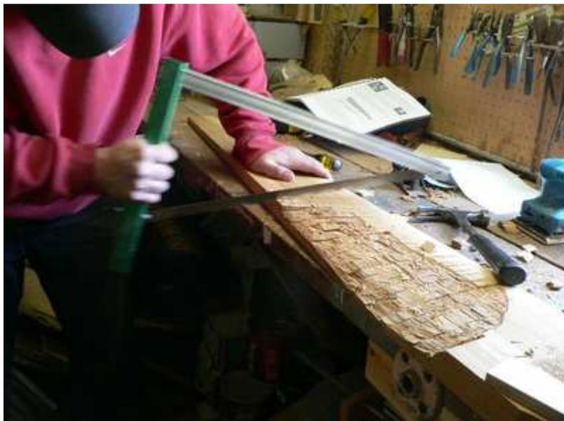
**A bow saw turned out to be an easy way to make the straight, deep kerfs at the blade roots**
