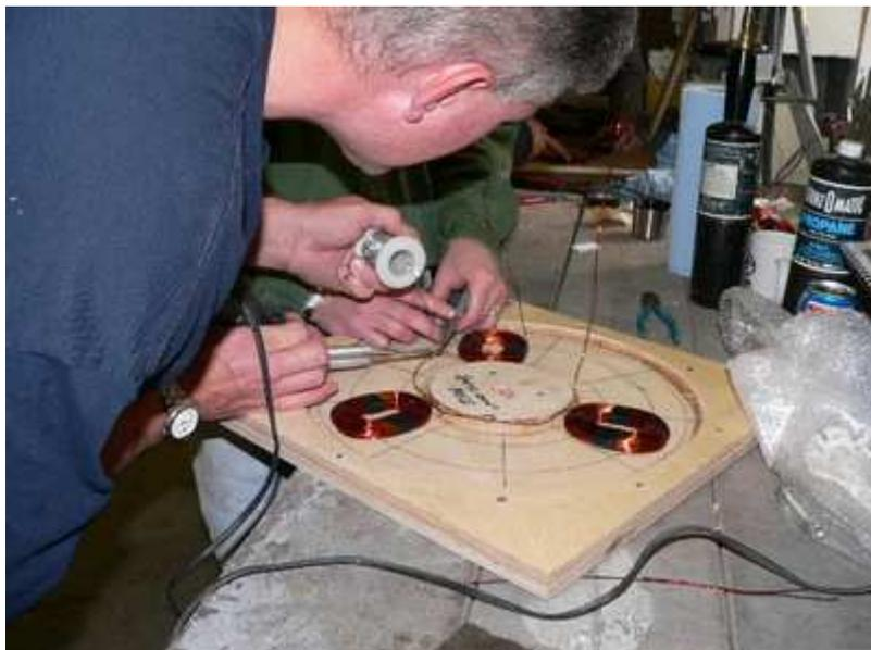
**Wiring one phase of the stator.**
