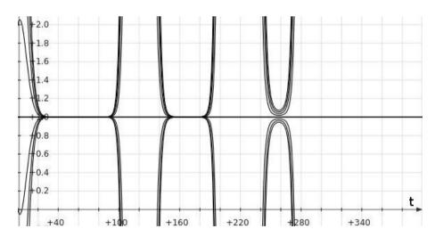
We will test now with softer reinforcements of the feedback. So, increasing slightly the negative feedback with  $y' = (1-y) \cdot (\sin(\frac{60 \cdot t}{1250 - t}) + 0'01)/2$  we get
