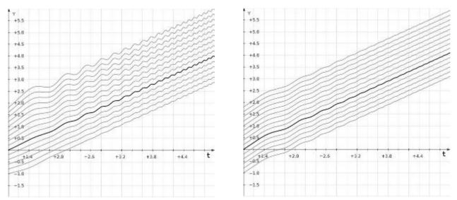
In this case, we see that the solutions of the differential equation  $y'=1+y\cdot\sin(t^3)/2$  are similar to the solutions of the equation  $y'=1+\sin(t^3)/2$ , only with greater oscillations. The reason of theses oscillations is precisely the feedback of y over y'. But, so that  $\sin(t^3)$  changes quickly of sign, as is showed in the following figure, the positive and negative feedbacks are succeeded and compensated without to arrive to predominate.
