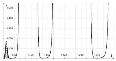
In this case, the curves converge after the first negative feedback, and this convergence keeps through the successive positive feedbacks.
