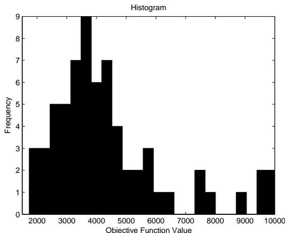
Figure 6: Histogram of solutions obtained from the multistart procedure for the integrated design and control problem
