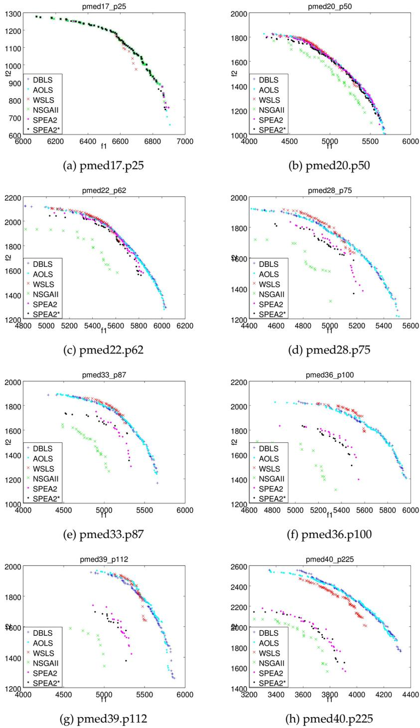
Figure 6: Non-dominated on 30 runs. NSGA-II and SPEA2 using their iRace configurations, and the rest of them limited to approximately the same number of evaluations.
