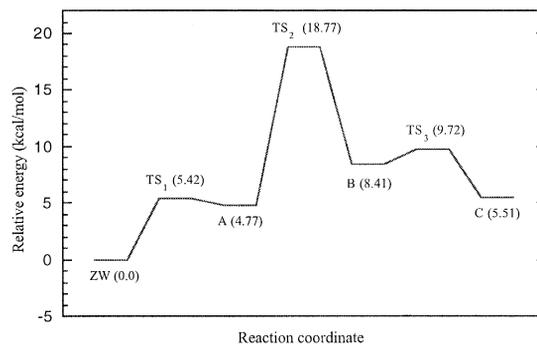
Fig. 4. Computed free energy profile for the tautomerization process of glycine in water.
