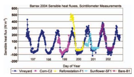
Figure 4. Sensible heat flux in SPARC 2004 (measurements made with scintillometers over different fields. See tables 1 and 2 for field code).
