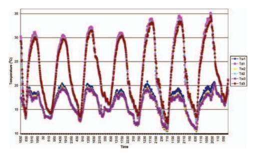
Figure 9. Air temperature and humidity measured at three levels. Tw is the wetbulb and Td the drybulb temperature; Tw1 and Td1 were set at a height of 0.65 m, Tw2 and Td2 at 1.65 m, and Tw3 and Td3 at 3.0 m.
