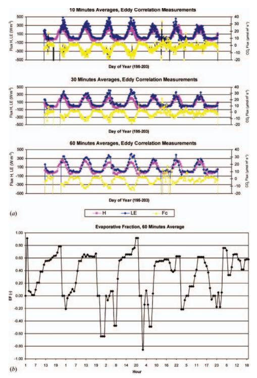
Figure 5. (a) Time-averaged sensible heat flux (H),  $H_2O$  (LE) and  $CO_2$  (Fc) fluxes and (b) time-averaged evaporative fraction (EF) measured with the eddy correlation station in SPARC 2004.
