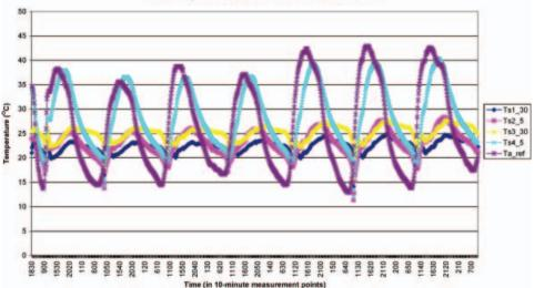
Figure 8. Soil temperatures measured with thermal couples at two levels in SPARC 2004. Ts1\_30, Ts2\_5, Ts3\_30 and Ts4\_5 are 30, 5, 30 and 5 cm below the surface, respectively; Ts1\_30 and Ts2\_5 are under the vine, while Ts3\_30 and Ts4\_5 are in the middle of the row; Ta\_ref is the reference air temperature measured at the eddy correlation station as shown in figure 5.
