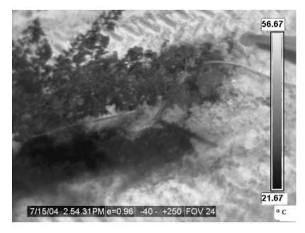
Figure 12. Radiometric temperature of the vineyard measured with an FLIR thermal camera in SPARC 2004. The spatial dimension of the image is approximately  $8 \text{ m} \times 6 \text{ m}$ .
