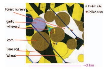
Figure 1. Locations of flux measurements in SPARC 2004. The base station of the scintillometer and the eddy correlation station were located in the vineyard during the complete campaign period. Other stations were installed for a limited period at different locations.
