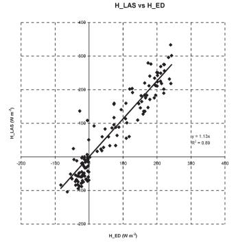
Figure 15. Scatter plots of sensible heat fluxes measured by the eddy correlation system and the scintillometer system with 60-min average in SPARC 2004.
